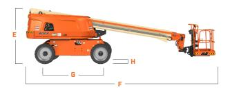
Platform Width 36-in / 0.91-m A. Platform Length 96-in / 2.44-m B. Machine Width C. 8-ft 2-in / 2.48-m D. Tailswing 4-ft / 1.22-m E. Machine Height 8-ft 2.4-in / 2.50-m F. Machine Length 28-ft 7-in / 8.71-m G. Wheelbase 8-ft 2.7-in / 2.5-m **Ground Clearance** H. 11.3-in / 29-cm
