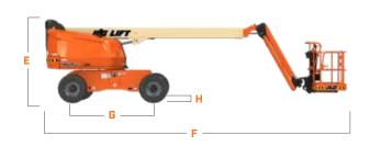
Platform Width 36-in / 0.91-m Platform Length 96-in / 2.44-m B. Machine Width 7-ft 6.8-in / 2.31-m C. D. Tailswing 2-ft 10-in / 86-cm E. Machine Height 8-ft 1-in / 2.47-m Machine Length F. 24-ft 11-in / 7.6-m Wheelbase G. 7-ft 9.5-in / 2.37-m Н. **Ground Clearance** 12.1-in / 31-cm
