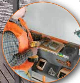
An optional 12V plug is connected to the scissor batteries to provide power to the customer-supplied tool or phone charger.
