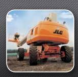
**Solid Ground** 45% gradeability and oscillating axle for improved traction.
