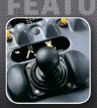
Lift/Swing Multiple use of control—lift and swing can be operated simultaneously.
