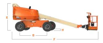
Platform Width 36-in / 0.91-m A. В. Platform Length 96-in / 2.44-m Machine Width C. 7-ft 6.8-in / 2.31-m 2-ft 10-in / 86-cm D. Tailswing Ē. Machine Height 8-ft 1.4-in / 2.47-m Ē. Machine Length 24-ft 10.1-in / 7.57-m G. Wheelbase 7-ft 9.5-in / 2.37-m **Ground Clearance** 12.1-in / 31-cm
