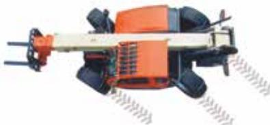
Crab steer for sideways movement and precise positioning before lifting.
